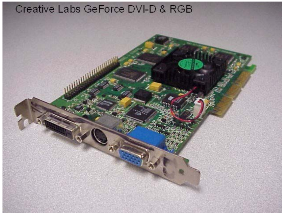
Photo 3, Typical AGP Video Card with DVI and VGA support
